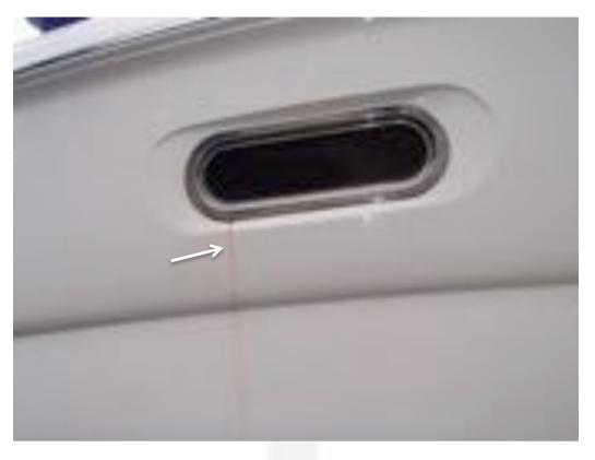
Image of the starboard forward portlight. Note the rust streaking.
