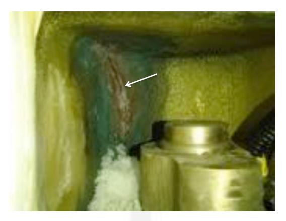
Image of the port stock and surrounding alloy cover. Note the weep form a suspected split in the cover.
