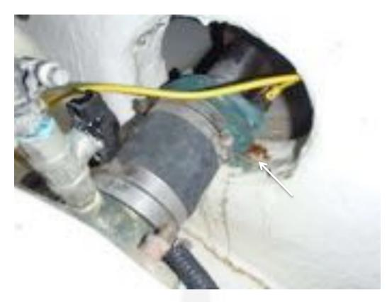
Port shaft seal. Note the surface corrosion developing and weep at the base.
